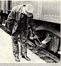
After every run, the engineer inspects his engine carefully, oils and tightens all major parts (left). Journal inspections are routine "musts" (above).
