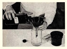
No. 5: While film is developing, filter correct amount of hypo, after rinsing funnel and jar a second time. Give tank a twirl occasionally. Adjust hypo temperature to same warmth as developer, or at least within one or two degrees, by immersing jar in hot or cold water, as required.
