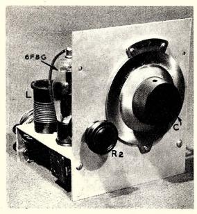
Above—A front view showing the position of the two controls. If a smaller dial is used for the tuning control (C), the panel size can be reduced. Right—The rear view of the receiver shows the simple arrangement of the parts. Metal construction is used throughout.
