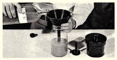
No. 2: Filter amount of developer required by tank, using wad of cotton in large funnel. Old fruit jar better than bottle; supports funnel more securely. Adjust developer temperature by immersing jar in hot or cold water. Most formulas call for 65 degrees F.
