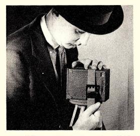
ATTACHING BOX CAMERA TO TRIPOD. When the lens aperture of a box camera is stopped down, and time exposures used, the results frequently are as good as can be obtained with a more expensive camera. The camera can be mounted securely to the tripod with a luggage or book strap.
