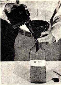
No. 6: After developing time has elapsed, pour developer back into bottle, using thoroughly rinsed funnel. Most finegrain developers can be used over and over if kept in tightly corked bottles. Screw caps are better than ordinary corks; latter tend to jump out if bottle is full.
