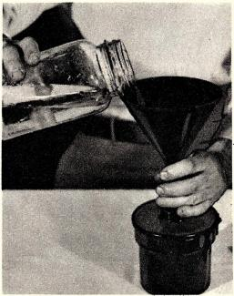
No. 9: After tank is drained of water, pour in hypo (previously filtered). Pour slowly to prevent splashing. Note time. Leave hypo in 15 minutes; this is standard regardless of type of film or developer.
