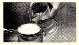
FILTERING DEVELOPER QUICKLY. When time must be saved, solutions can be filtered quickly by using a nickel-wire strainer lined with a layer of cotton. If the strainer is not nickel plated, it should be coated thinly with asphalt varnish.
