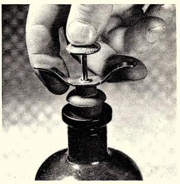
SEALING DEVELOPER BOTTLES. A rubber cork of the expansion type, used for bottles of charged water, is a convenient and efficient cork for sealing bottles of developer.
