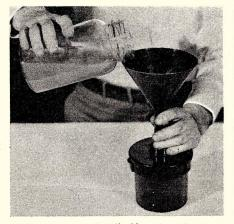
No. 3: Rinse funnel well. Note time, then pour in developer slowly, giving air plenty of time to escape. Rinse funnel and jar thoroughly, invert on sink to drain.
