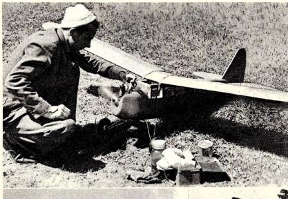
Left—Many a contest is won in the "pits", the roped off areas where the modelers are permitted to adjust the miniature gasoline engines of their entries. The adjustment of the carburetor needle-valve often means success or failure of the flights.
