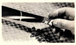
PREVENTING CURLING OF ROLL FILMS. Unless roll films are prevented from curling while in the hypo solution, portions may not become thoroughly fixed. Films will lie flat in a tank if the ends are fastened together with small clips as shown above.
